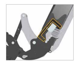
The steel sections have five edges and the cross beam is double-walled, providing a torsion-free structure that withstands the toughest conditions. The cross beam is mounted at an angle to adopt the operator's line of vision for best visibility.
