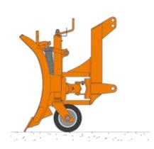
When the cutting edge hits an obstacle such as a gully, the overload mechanism trips and the blade moves up. At the same time its base moves to the rear, floating over the obstacle. Return springs return the blade into working position after the tractor has been halted or the blade raised. The tripping force is set steplessly to suit individual snow and ground conditions and the application at hand.
