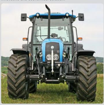
The inclined lower control arms are situated closely to the front linkage during folding-up.
