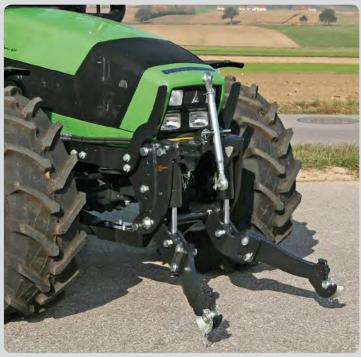
Combination attachment parts with snow plough coupling plate: The universal capability of the "FS-4" is evident by the possibility of mounting a snow plough coupling plate to the combination attachment parts when front linkage is removed.
